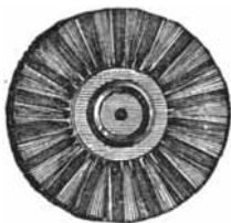
FIG. 32. CIRCULAR SCRATCH BRUSH. MADE OF WIRE OR OF BRISTLES.
