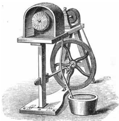
FIG. 36. FOOT-POWER SCRATCH-BRUSH LATHE.
